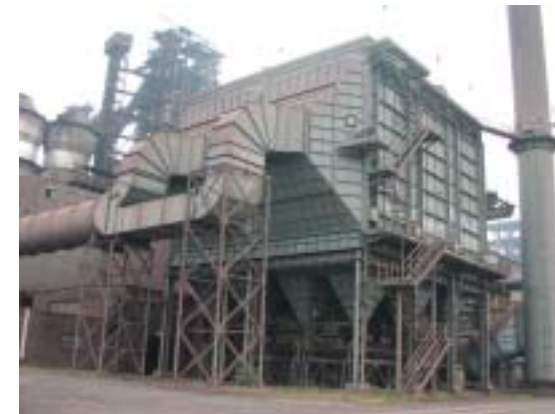
VP3 Elektroodlučovač s opacimetrom Blast Furnace #3 Electrostatic Precipitator with Opacimeter
