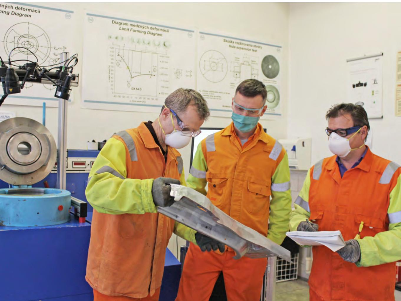
(Erichsen tester, Impact tester, bend tester, coating adhesion tester using the grid method), used to simulate the material's behavior during its processing by our customers.
